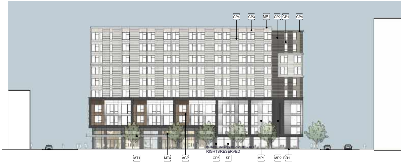
2 OVERALL WEST ELEVATION 3/64" = 1'-0"
