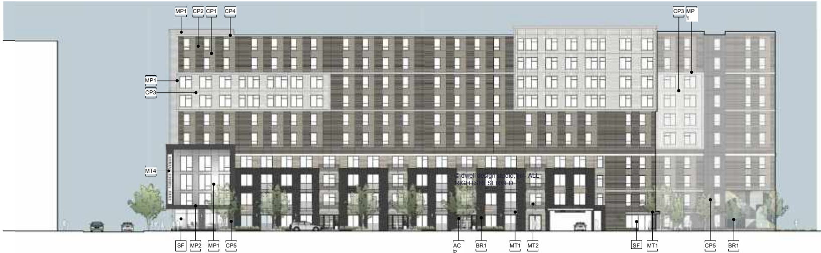
1 OVERALL SOUTH ELEVATION - MCKEE PL. 3/64" = 1'-0"
