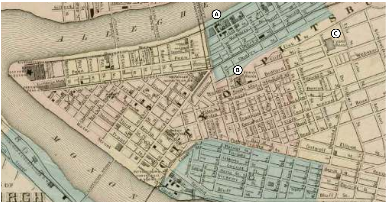
Figure 50. Detail from The Cities of Pittsburgh and Allegheny, with Parts of Adjacent Boroughs , 1855, showing Pittsburgh's expanded water supply system. Water was drawn from a new intake on the Allegheny River (A) then pumped to the Lower Basin (B) and the Upper Basin (C) in the Hill District (Historic Pittsburgh).
