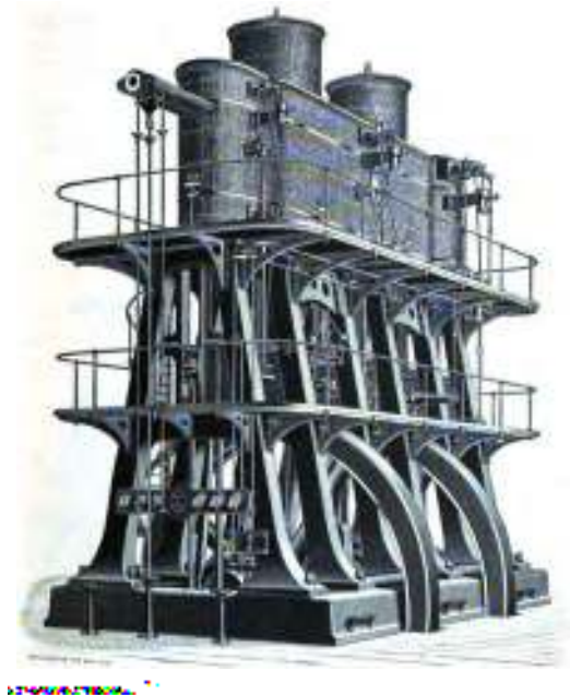
Figure 54C. Perspective drawing of just the engine component of an Allis triple expansion pump. This would have been similar to the equipment visible through the windows on the first floor of the Herron Hill Pump House ("American Inventors: Elisha Gray," The National Magazine , May-June 1893, v. 18, no. 1, 65).
